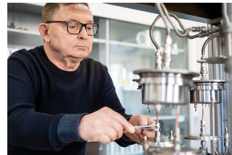
> Pumping units for evacuation of air and filling the ionisation chambers with noble gas
