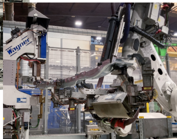
Automatic setting of weld nuts in the assembly cell
